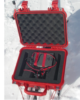
Radar Transmitter and carrying box mounted on skis. Photo Credit: Laurent Mingo
